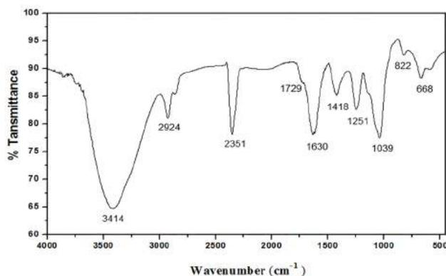
**Figure 1:** Infrared spectrum of the FCS.
