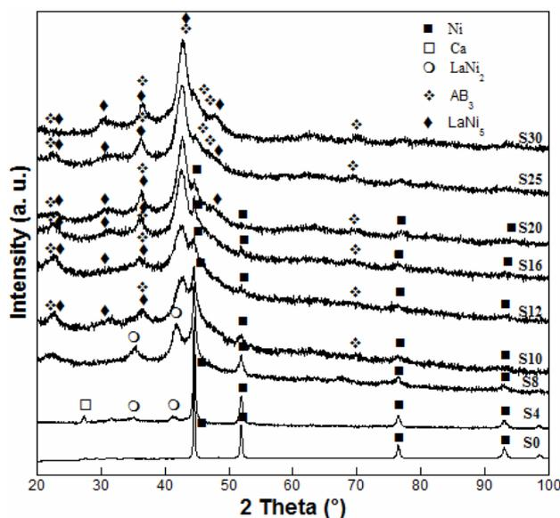
**figure 1:** Evolution of the XRD patterns of samples for increasing MA duration (4 to 30 hours).
