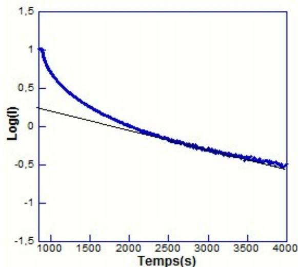
figure 8: Semilogarithmic plots of anodic current-time responses of the S30 sample.
