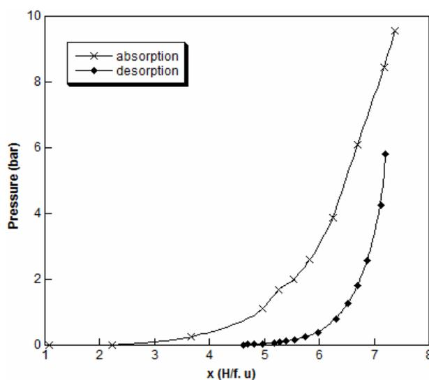
**Fig. 5 :** PCT curve of the S30 sample measured at 25 °C [13].
