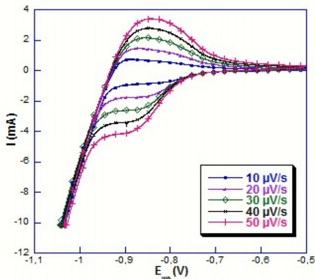
figure 6: Cyclic voltammograms of S30 sample at potential scan rate: 10, 20, 30, 40 and 50 μV/s.
