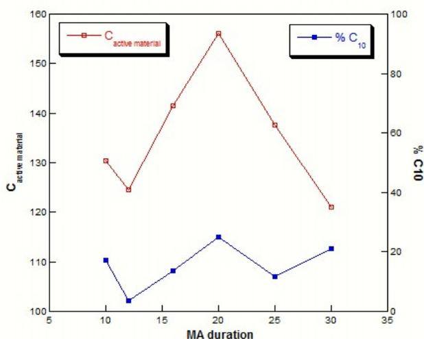
**figure 4:** Effect of MA duration on the discharge capacities of the active material at the first cycle and the loss of discharge capacity at the 10<sup>th</sup> charging-discharging cycle.
