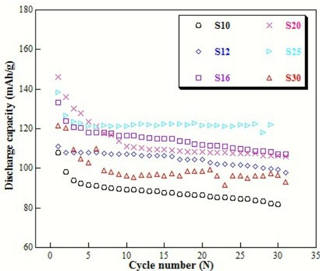
figure 3: Variation of the discharge capacity vs cycle number of S10 to S30 samples
