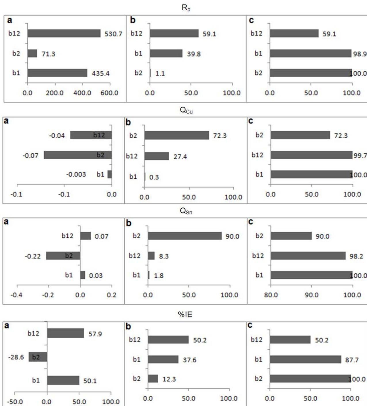
**Fig.4:** (a) The estimated model coefficients, (b) Pareto charts and (c) cumulative Pareto charts for the different electrochemical responses
