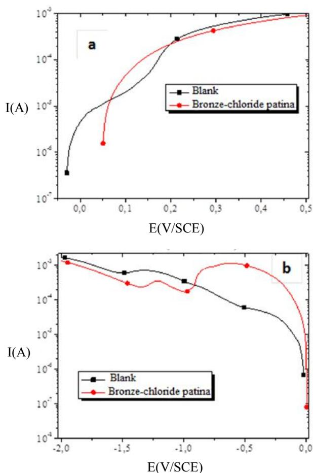
**Fig.2:** The I-E curves of the bronze electrode immersed for five minutes in  $1\text{g.L}^{-1}$   $\text{Na}_2\text{SO}_4$  solution without and with the patina layer (a) anodic range, (b) cathodic range, the scan rate fixed at  $1\text{mVs}^{-1}$ .
