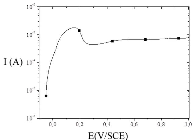
**Fig.1:** The anodic polarization curve of the Cu10Sn bronze alloy immersed for one hour in 0.1M NaCl solution, at a scan rate fixed at  $1\text{mVs}^{-1}$ .
