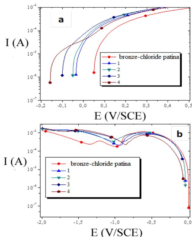
**Fig.3:** Polarization curves of the patinated bronze in the presence of the extract according to the experimental design (a) anodic range, (b) cathodic range. Scan rate fixed at  $1\text{mVs}^{-1}$ .
