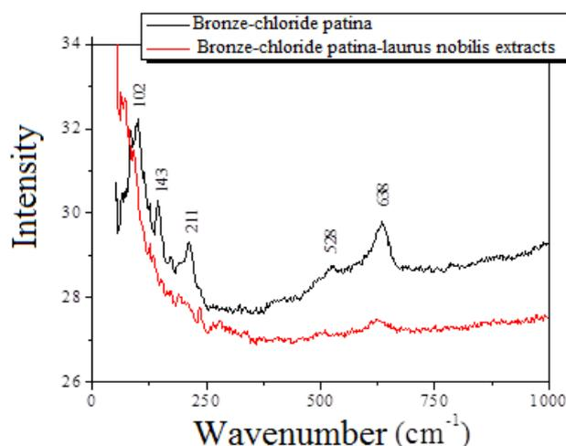
Fig.5: Raman spectra of patinated bronze without and with the extract addition
