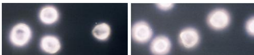
Fig. 7: Optical texture (x200) of 3a at 95°C observed on cooling from isotropic liquid Fig. 8: Optical texture (x200) of 3b at 130°C observed on cooling from isotropic liquid
